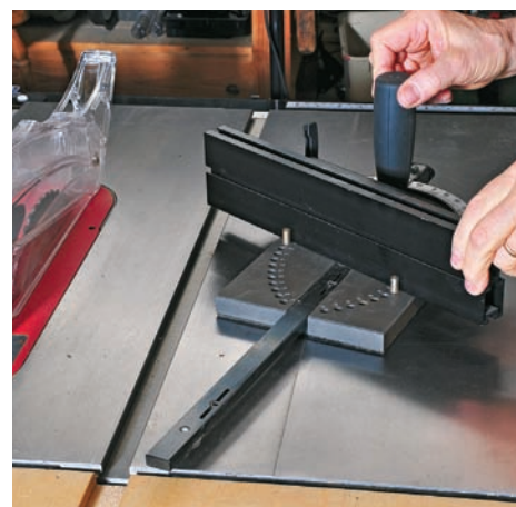
Simple and accurate. Pins inserted into a plate are a precision reference for the miter gauge’s fence. It takes no time to set up the jig, slide the gauge into place, and lock in the fence’s angle.
