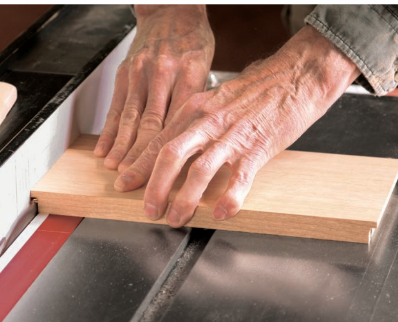
Creating the lip. A rabbet is cut on three sides (left), and a profile is routed (above), planed, or scraped into the lip.
