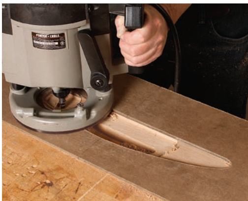
Second template. Align the centerline of the second template with the centerline of the rail. Then use a router and short flush-trimming bit to relieve the area down to a depth of about ⅛ in. (above). Add the texture using a carving gouge (right).
