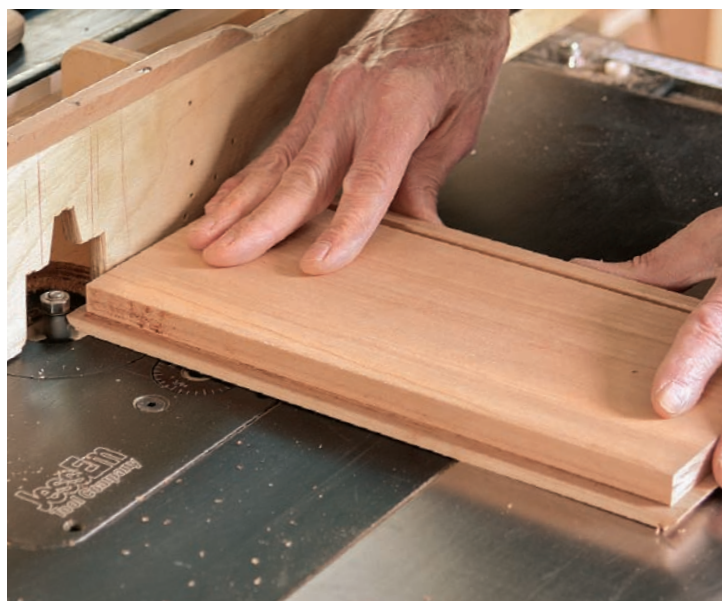
Creating the lip. A rabbet is cut on three sides (left), and a profile is routed (above), planed, or scraped into the lip.
