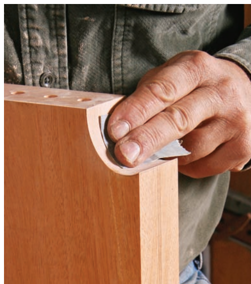
Filed fair. Files and sandpaper combine to fair the bandsawn curve (above). A half-round file and handheld sandpaper smooth out the tight cutout at the shoulder of the leg (left).
