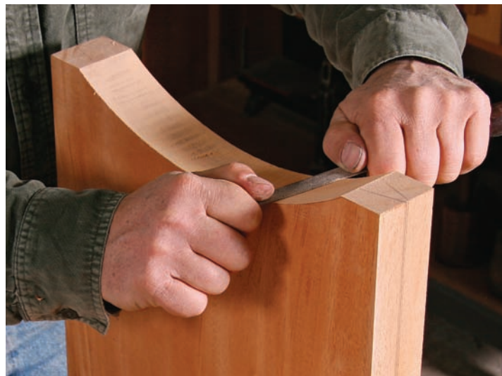
Filed fair. Files and sandpaper combine to fair the bandsawn curve (above). A half-round file and handheld sandpaper smooth out the tight cutout at the shoulder of the leg (left).
