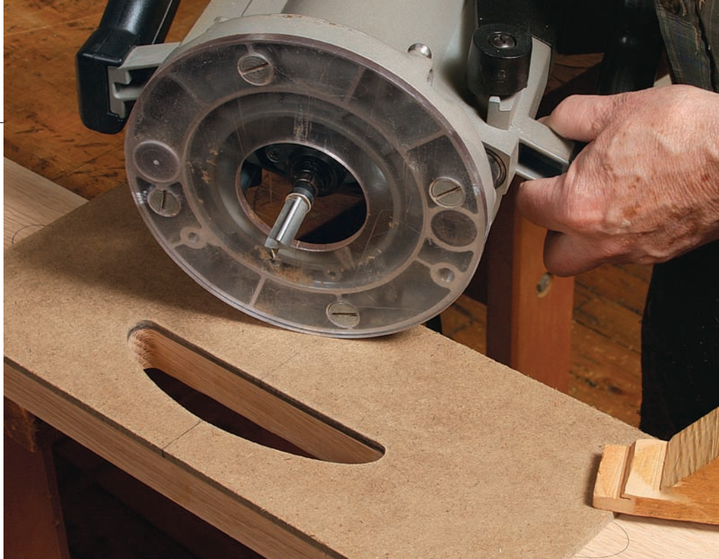
First template. Use a ¼-in.-thick Masonite template to lay out the through-cut. Then rough it out with a jigsaw (above). Use the template and router with a flush-trimming bit to finish the work (right).
