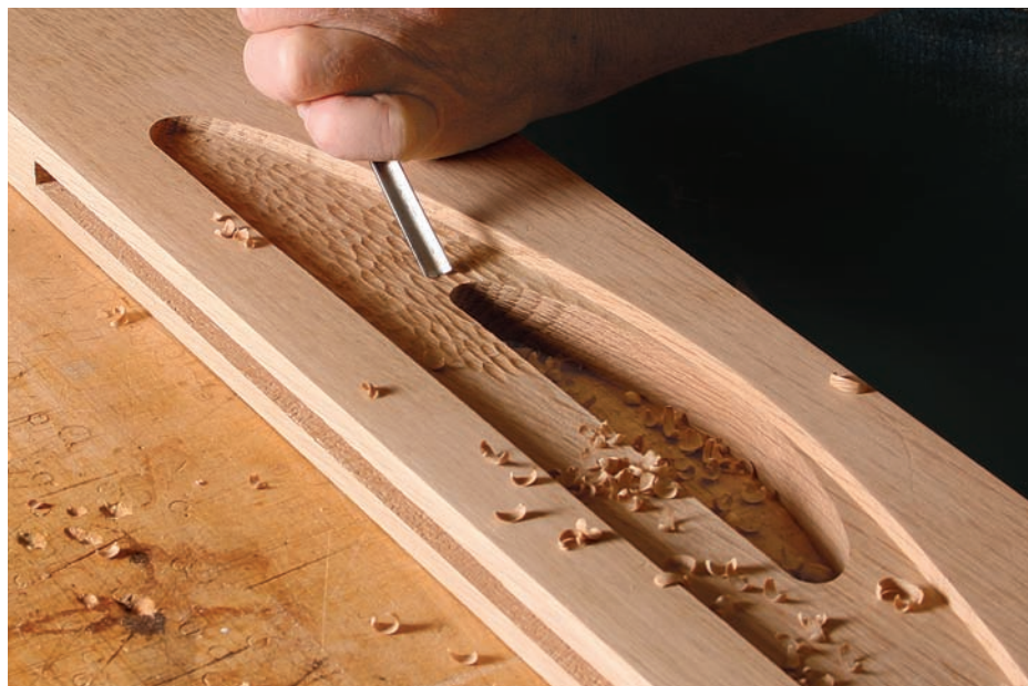
Second template. Align the centerline of the second template with the centerline of the rail. Then use a router and short flush-trimming bit to relieve the area down to a depth of about ⅛ in. (above). Add the texture using a carving gouge (right).
