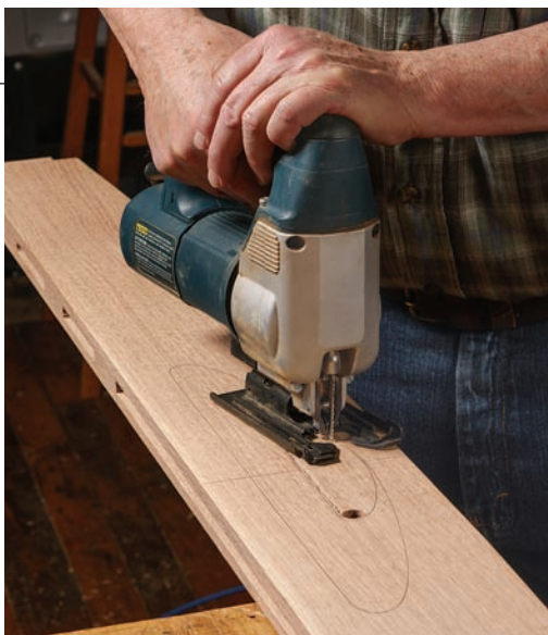
First template. Use a ¼-in.-thick Masonite template to lay out the through-cut. Then rough it out with a jigsaw (above). Use the template and router with a flush-trimming bit to finish the work (right).
