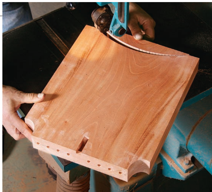
Saw out the foot scoop. The bandsaw makes quick work of cutting the curved cutout at the base of the leg.
